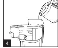
Lift lid and pour water from carafe into reservoir. NOTE: Do not fill past the 12-cup mark (60 ounces [1.8 L]).
