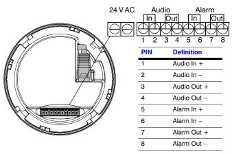
3. Connect a twisted pair (UTP) cable from each peripheral alarm contact to each alarm input on the terminal block. For detailed audio and alarm configuration information, refer to the appropriate user guide located on your software DVD.
