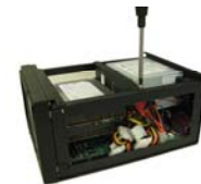
6. Fix the HDD bracket into the internal unit.
