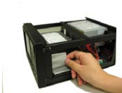
7. Connect HDD cable to IDE port.
