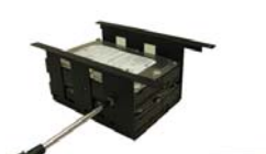
5. Install the second HDD on the bracket.
