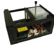
3. Dismantle the HDD bracket.
