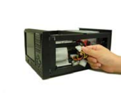
8. Connect power cord to the HDD.
