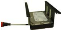
4. Install the first HDD. Note the HDD is placed upside down. Please make sure bracket is in correct position.
