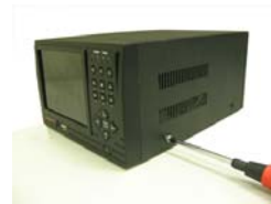
9. Place the unit cover back and screws firmly.
