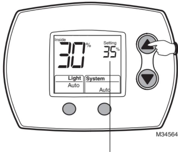
The humidity setpoint will flash if the humidity control is waiting for the dehumidifier protection time to run out.
