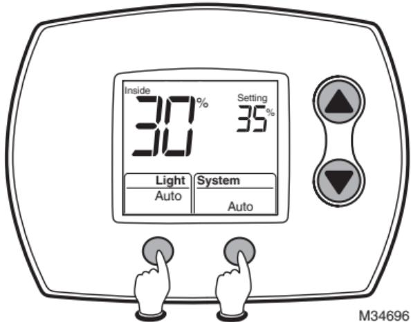
To begin, **press and hold** the **SYSTEM** and **LIGHT** buttons until the display changes.
