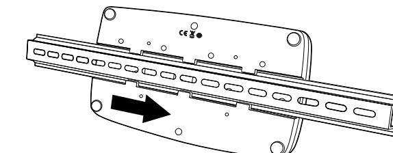
2. Then, using the appropriate hardware above, secure the DIN rail to the desktop.
