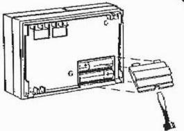
Re-assemble the unit and switch on the mains supply. The clock is reset to Mo (Monday) 12.00 pm and the built in programme is re-established.
