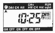
NOTE: If no adjustment is made for five minutes the Programmer resumes automatic operation. To indicate this, an arrow appears below at the top right of the display.
