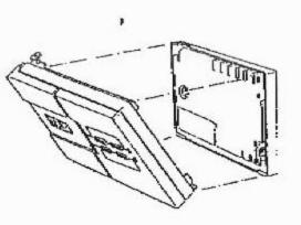
Release the cover by inserting a small screwdriver, nailfile or similar tool into the slot at the bottom and lever it up.
