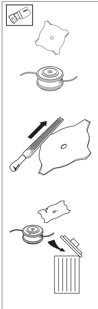
2) Keep the blade's teeth well and correctly sharpened! Follow our instructions and use the recommended filing gauge. An incorrectly sharpened or damaged blade increases the risk of an accident.
