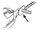
Check that the hand guard is fitted correctly.
