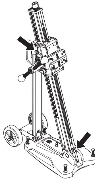
Loosen the locking screws for column tilt and set the desired drill angle. Tighten the locking screws. Use the feed lever. The column can be tilted 0-60°.
