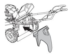
3 Close the back shield to allow the machine to discharge material to the left of the machine while cutting.
