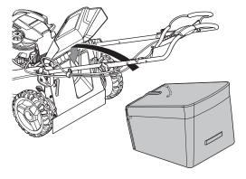
3 Release the back shield and allow it to rest on top of the grass bag frame.
