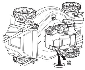
6 If you have spilled fuel or engine oil on the machine, wipe off the spillage and allow remaining fuel to evaporate.
