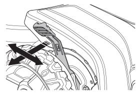
• The adjuster lever is spring loaded.
