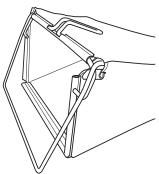
2 Secure the grass bag to the frame by using the quick-action clips.
