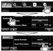
Touch the center of the marks at the lower left and at the upper right as instructed.
