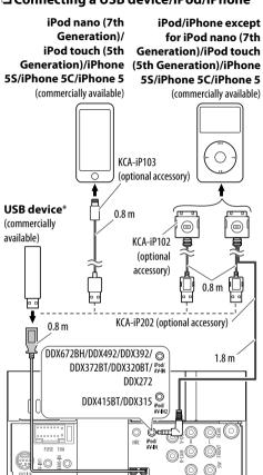
\* Use CA-U1EX for extending the cable if necessary. (Max 500 mA, 5V)
