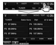
The preset list containing the station names for FM RBDS (when a PS signal is coming in) is displayed.
