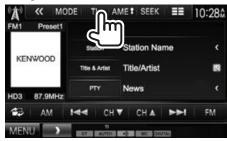
The unit is in standby to switch to Traffic Information (TI) if available. (The TI indicator lights up in white.)
