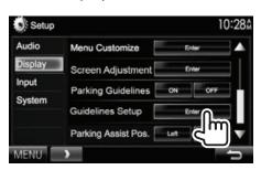
**3** Adjust the parking guidelines by selecting the 器 mark (①), then adjusting the position of the selected the mark (2).
