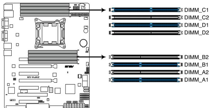
**Z9PA-U8 240-pin DDR3 DIMM sockets**
