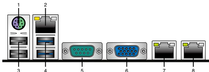
1. **PS/2 mouse and keyboard port.** This port is for a PS/2 mouse and keyboard.
