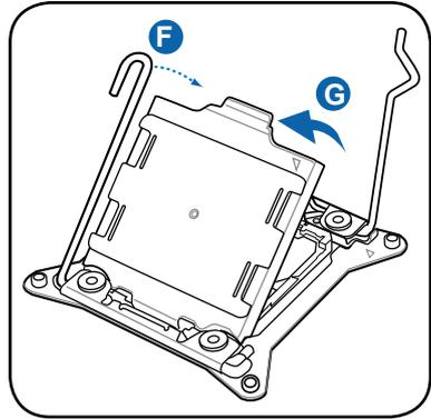
6. Position the CPU over the socket, ensuring that the triangle mark is on the top-right corner of the socket.
