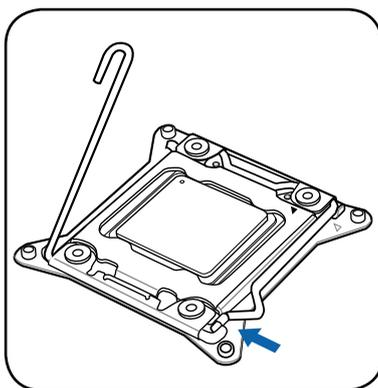
10. Push down the left load lever (L), and then insert the lever under the retention tab (M).
