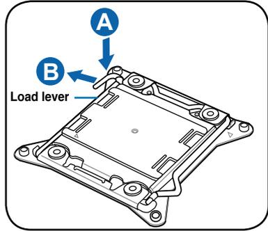
3. Slightly lift the load lever in the direction of the arrow.
