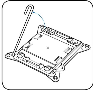
4. Press the right load lever with your thumb (C), then move it to the right (D) until it is released from the retention tab. Lift the load lever in the direction of the arrow (E).
