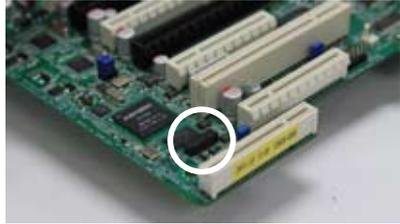
2. Orient and press the ASMB6 management card in place.
