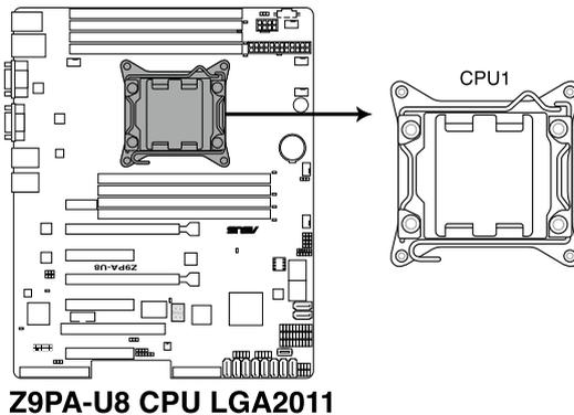
2. Press the left load lever with your thumb (A), then move it to the left (B) until it is released from the retention tab.
