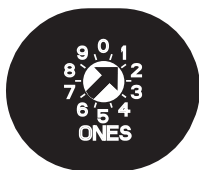
Figure 3.1: Address switch set to 1
