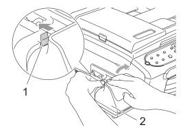
4 Pull the tab (1) back and hold it in position as you push the bracket (2) to the back of the machine.
