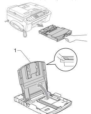
Press and slide the paper side guides (1) and paper length guide (2) to fit the paper size.
