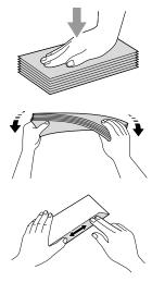
Put the envelopes or post cards into the paper tray with the address side down and the leading edge as shown in the illustration in first as shown in the illustration. Slide the paper side guides (1) and paper length guide (2) to fit the size of the envelopes or post cards.
