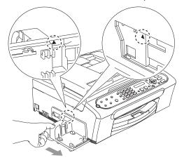
3 Make sure you plug the connector into the jack (1) and route the cable through the hook (2) as shown below.
