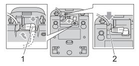
4 Press the tab (1) and place the front of the cradle in position.
