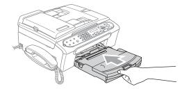
8 While holding the paper tray in place, pull out the paper support (1) until it clicks and unfold the paper support flap (2).
