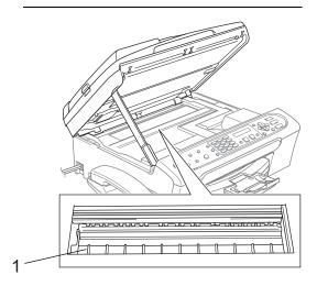
1 Clean the machine printer platen (1).
