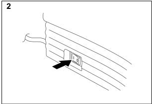
Turn on the power switch that is located on the left side of your printer.
