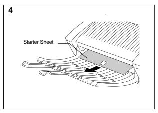
Make sure that the printer automatically ejects the starter sheet while the printer is warming-up immediately after installing a new drum unit. You may discard the starter sheet after it is automatically ejected.
