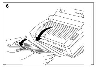
Open the output tray. (①) Extend the extension support wire. (②)
