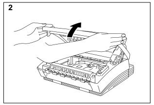
Open the top cover of the printer. Make sure that the cover is correctly latched open, indicated by a click.
