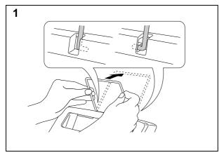
Install the paper support onto the multipurpose sheet feeder.
