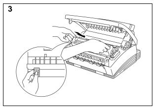
Holding the drum by its handles, install it into the printer.
