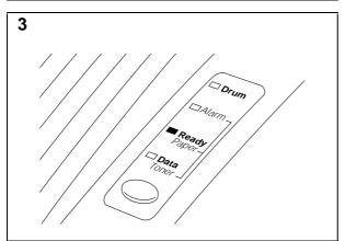
Make sure that the READY lamp is lit after the printer has warmed up (approximately 20 seconds).
