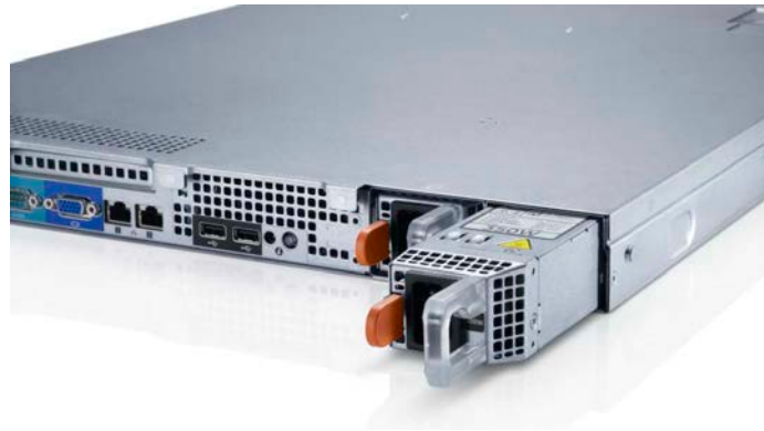
Figure 7. 350W power supply unit
