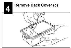
Carefully pull up each side of the REAR HOUSING cover until it is completely removed.
