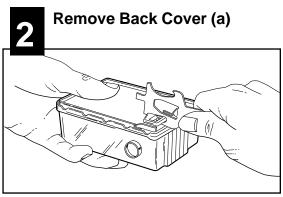
Insert special tool into rectangular hole of PULL TAB.
