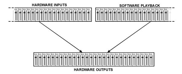
56 channels don't fit on the screen side by side, neither does such an arrangement provide a useful overview. The input channel should be placed above the corresponding output channel. Therefore, the channels have been arranged as known from an *Inline* desk, so that the row *Software Playback* equals the *Tape Return* of a real mixing desk:
