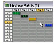
To maintain overview when the window size has been reduced, the left and upper labels are floating. They won't left the visible area when scrolling.
