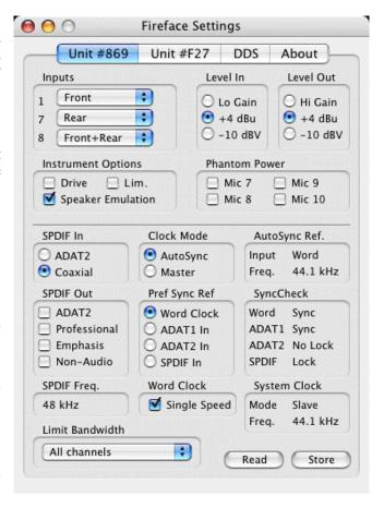
At 88.2 or 96 kHz: If the ADAT input has been selected in *Pref Sync Ref*, the sample frequency shown in the *SPDIF Freq.* field differs from the one shown in *AutoSync Ref.* The unit automatically switches to S/MUX mode here, because ADAT optical inputs and outputs are only specified up to 48 kHz. Data from/to a single input/output is spread over two channels, the internal frequency stays at 44.1 or 48 kHz. In such cases, the ADAT sample frequency is only half the SPDIF frequency.
