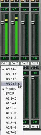
Please set Out 4 to a gain of around -20 dB and the pan close to center. Now click onto the routing field. You'll now see two checkmarks, one at 'AN 3+4', the other one at 'AN 7+8'. Click onto 'SPDIF'. The window disappears, fader and pan jump to their initial values, the signal can now be routed to the SPDIF output. You can continue like this until all entries have got a checkmark, i. e. you can send the signal to all outputs simultaneously.
