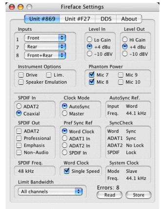
The string **Errors** is displayed only when transmission errors of PCI/FireWire are detected. The display will be reset on any start of a playback/record, i.e. set to zero and is thus no longer visible. More information can be found in chapter 37.3.
