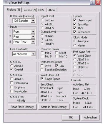
whether there is a valid signal (Lock, No Lock) for each input (Word Clock, ADAT1, ADAT2, SPDIF), or if there is a valid *and* synchronous signal (Sync). The *AutoSync Ref* display shows the input and frequency of the current sync source.
