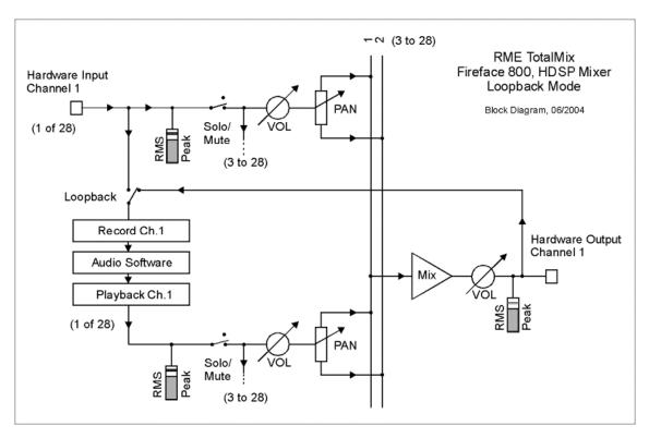
As each of the 28 hardware outputs can be routed to the record software, and none of these hardware inputs get lost, TotalMix offers an overall flexibility and performance not rivaled by any other solution.
