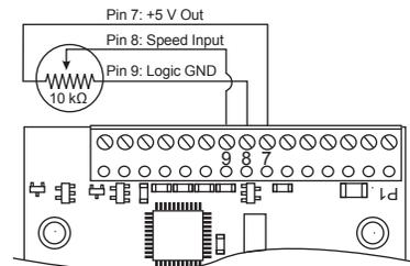
The Analog Speed Control Input may be connected on any device with a 0 to +5 VDC output such as a sensor
