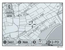
**F3 (Heading)** – Changes the map heading between north to the top of the screen and vehicle heading to the top of the screen.
