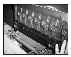
Remove the driver's and passenger's side folding floor extensions.
