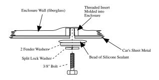
**STEP 8:** While one person holds the Stealthbox in place from above, the other person inserts the bolt, lock washer and fender washers from underneath the vehicle. Put a bead of silicone sealant between the car's sheet metal and the fender washers.
