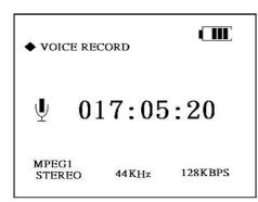
Press  $\blacktriangle \blacktriangledown$  button to select recording function in the main menu and use  $\hookleftarrow$  to enter.
