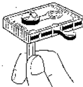
Figure 6. If tape is pulled out, use a pencil (as a spindle) to pull it back into shell.
