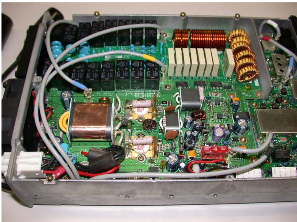
Fig. 5: 100W final section with antenna tuner
