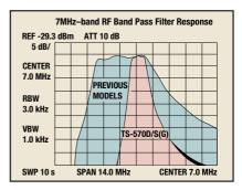
(one each for high band and low band) allow you to select better sensitivity or higher IMD performance, and the dedicated 7 MHz and 14 MHz bandpass filters deliver improved SW intermodulation rejection.
