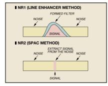
SPAC (Speech Processing by Auto Correlation) Method (NR2) for CW. The Line Enhancer Method automatically forms a filter shape around
