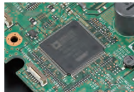
For band scope ADSP-21363 clock @333 MHz
