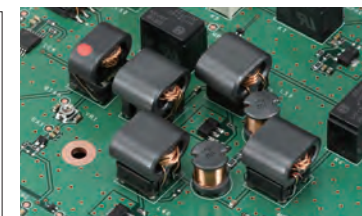
Transformer feedback RF Amp
