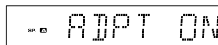
Appears for a few seconds after the adaptor input is turned on.
