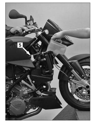
To completely bleed the cooling system, the motorcycle must be raised approx. 50 cm in the front.
