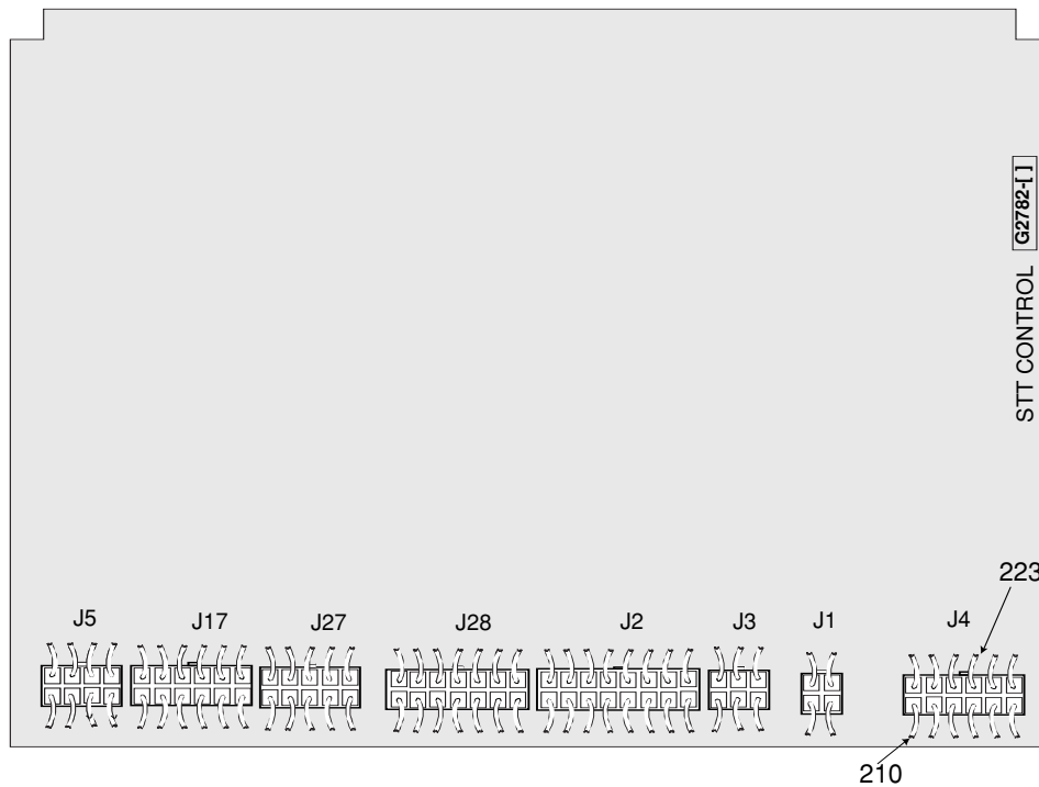
FIGURE F.21 – CONTROL PC BOARD MOLEX PLUG
