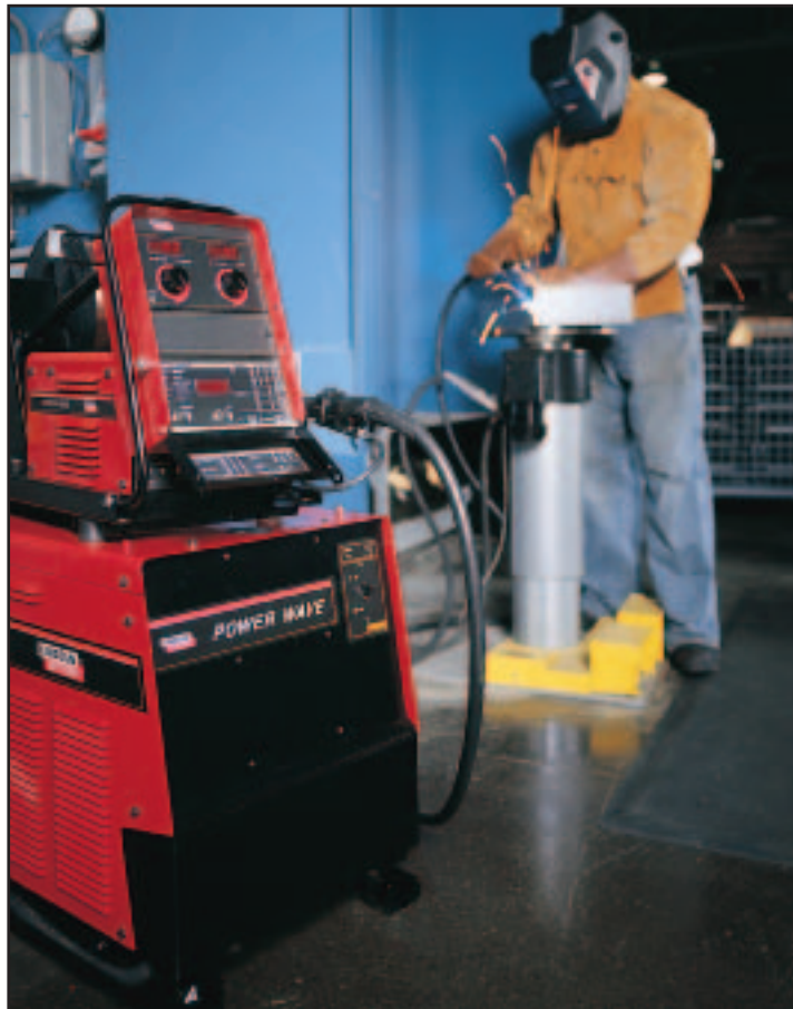
The Power Wave® 455M uses Inverter technology to produce consistent welds with a variety of weld processes.
