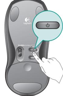
**English** Press and hold Power button for one second to turn ON mouse. Power LED glows green for 20 seconds.
