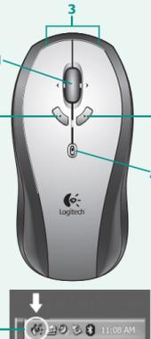
**English** 1) Tilt wheel plus zoom. Push wheel to either side to scroll horizontally. Click and roll the wheel to zoom in and out. (Works only if software is installed.) 2) Universal forward and back buttons. 3) Left and right mouse buttons. Launch Logitech® SetPoint™ to customize button and tilt wheel assignments. 4) Battery LED. LED glows green briefly when mouse is powered. LED blinks red when battery level drops below 10%.
