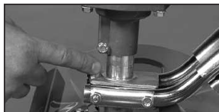
Picture 3. Note how the engine doesn't sit all the way down on the transmission.
