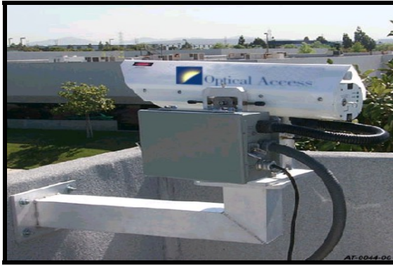
Figure 2.10: Extended Wall Mounting (using JMP and MO62C)
