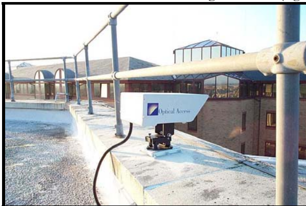
Figure 2.6: Parapet/Ledge Mounting (using JMP only)
