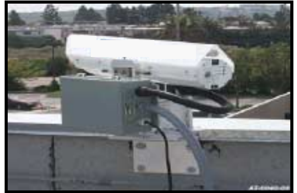
Figure 2.11: Angle Bracket Mounting (using JMP and M001)
