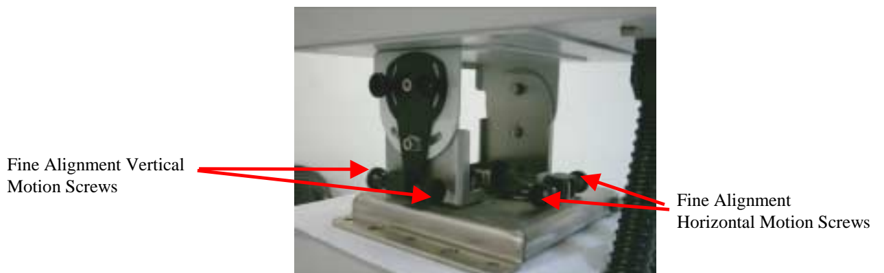
Figure 6.11: Fine Alignment Motion Screws
