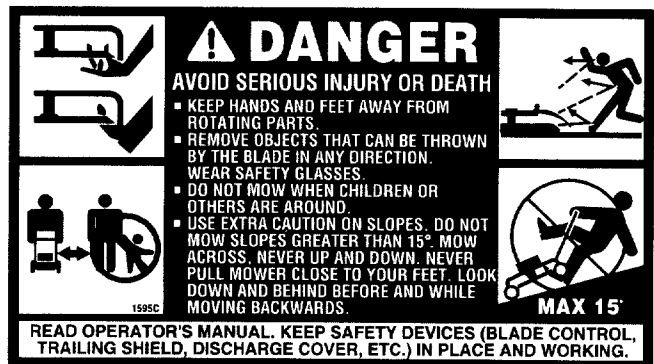
Figure 2 Safety Labels Found On Lawn Mower
