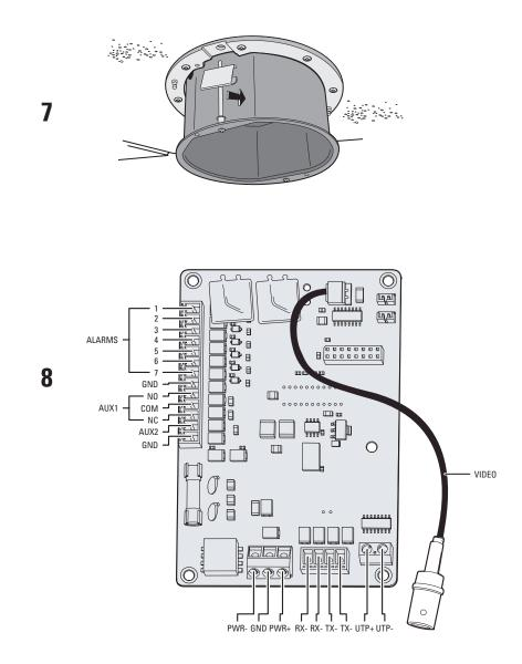
7. Install the back box by compressing the spring clips and pushing the back box through the hole. Tighten the screws until you hear a clicking noise.
