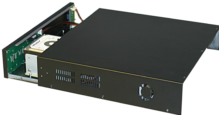
Figure 5. Removing the Top Cover
