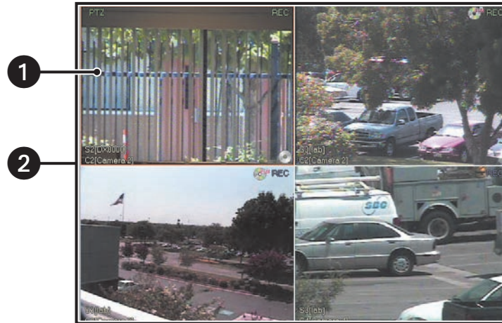
Figure 3. View Panes and Panel for 4-Division Display
