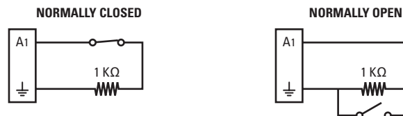
Figure 11. Supervised Alarm Input Wiring
