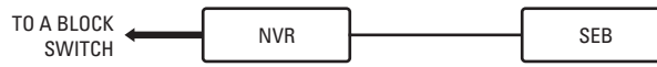
Figure 10. Using a Patch Cable to Connect the NVR5100 and a Single SEB5000
