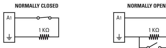
Figure 11. Supervised Alarm Input Wiring
