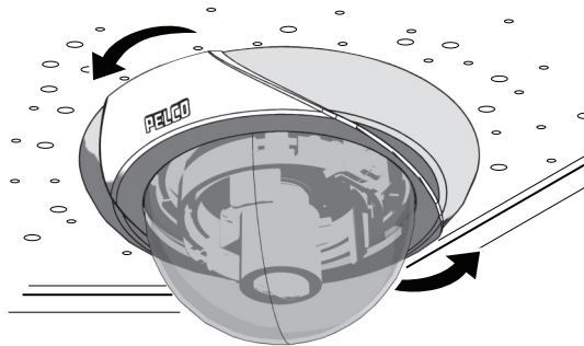
Figure 12. Positioning the Top Cover of the Lower Dome
