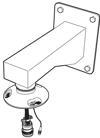
Thread the wiring from the mount through the mounting plate, and then attach the mounting plate to the mount. If outdoors, apply thread compound (provided) to the threads on the mounting plate.
