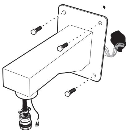
Feed a fiber optic cable (not supplied) and the supplied wiring harness into the front of the mount and out the back of the mount. Connect the wires as required. Refer to Tables A, B, and C for cable and wiring information. Fasten the mount to the mounting surface. Refer to the instructions supplied with the mount.
