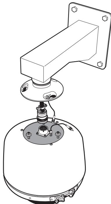
Attach the connector of the wire harness to the mating connector located on the top of the back box. Connect the fiber optic cable. Insert the studs and nuts on top of the back box into the mounting plate, turn the back box counterclockwise, and then tighten the three nuts.
