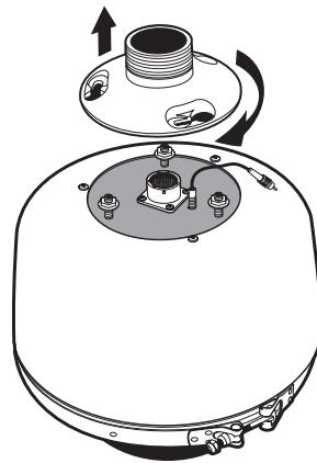
Remove the back box mounting plate: Loosen the nuts on top of the back box until they reach the locking material at the end of the studs, and then turn the mounting plate clockwise and lift.
