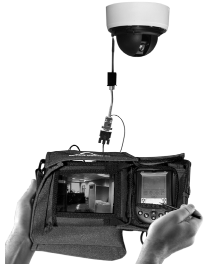
Figure 8. Remote Monitor Kit Connected to a Spectra Mini Dome
