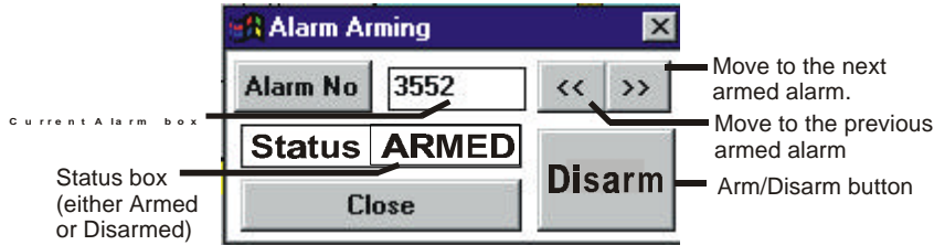
Figure 4-4: The Alarm Arming Window.
