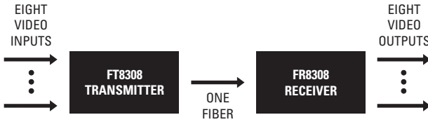
Figure 1. Eight-Channel Video FT8308 Transmitter and FR8308 Receiver
