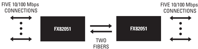
Figure 1. FX82051 Point-to-Point Application
