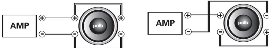
With coils in parallel, a dual 4 Ohm speaker will present a 2 Ohm load.
